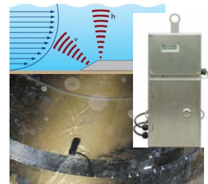
Measuring device for gravity lines
